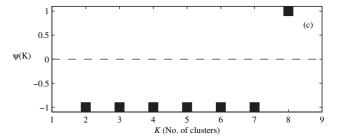
Figure 4. Clustering performance using similarity factor for the CSTR example. SF  $= 0.67 S_{\text{PCA}}^{\lambda} + 0.33 S_{\text{dist}}$ .
