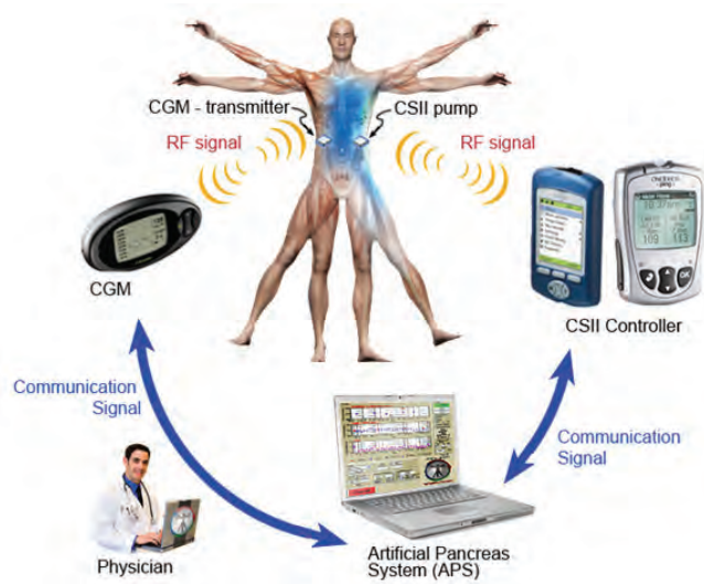
Schematic representation of closed loop artificial pancreas system.
